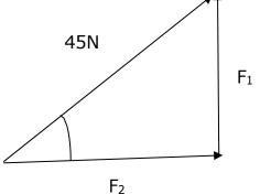
The resultant force of 45N is made up from two component forces  $F_1$  and  $F_2$ .
